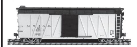
The Georgia RR and several other railroads chose to upgrade their USRA SS cars with steel plates welded to the inside of the bracing in place of the original wood. This was a quick and inexpensive method of obtaining an all steel car. It did not increase the interior capacity as much as the Youngstown sides and ends. AB brakes are included. "D" versions include a Georgia RR decal.
