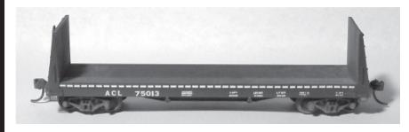
These cars were used to carry pulpwood (small diameter logs of no other commercial value that were used to make paper). They were converted from old flatcars by the addition of a steel deck sloped to the center and bulkhead ends. They were used by the ACL, SEABOARD, SOUTHERN and many other roads that had logging operations in their service area. "D" versions contain an ACL decal.
