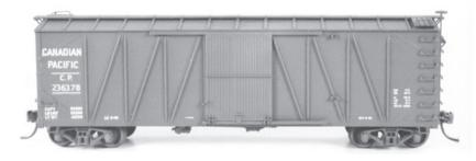
In 1921, the Canadian Pacific RR built a fleet of 3500 SS USRA copies. They were identical with the USRA standard except for the use of 7/8 ends instead of the 5/5/5 end. As built, they had grain unloading hoppers under the doors, but these quickly disapeared. This kit represents the post 1940 version with no grain doors, AB brakes, 7/8 ends and Bettendorf trucks. A CP decal is included.
