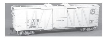
In 1934, the D&H converted 30 SS USRA boxcars to carry bulk cement with the addition of roof hatches, wine discharge gates and interior slope sheets. They were in the # series 17001 - 17500. The B&O also converted 40 cars numbered from 287000 - 287039. After 1960, these cars were used in company sand service with the D&H operating at least one into 1985. "D" versions include a D&H decal, see decal section for B&O decals.
