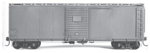
These cars were rebuilt during the late 30's through the 40's from USRA single sheath boxcars through the use of standard side assemblies supplied by the Youngstown Company. Includes both ribbed and non-ribbed extended ends. AB brake gear is included.
