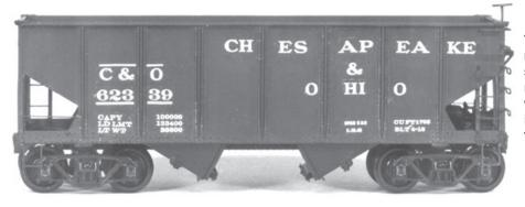
These all steel hoppers were the most enduring of all the USRA designs. 22,000 were built for 23 railroads. In addition, the basic design was adopted as standard by the ARA in 1922. Cars remained in service through at least 1972.
