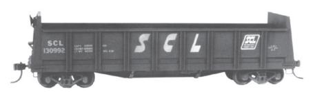
Both the ACL and the SCL converted pulpwood cars into stump cars. These were used used to haul stumps from logging operations to chemical plants that extracted chemicals from the pine tar in them. The conversion was done simply by using steel plates with a pair of angles reinforcing the top edge and channels for vertical support. The gap between the plates and the deck allowed debris to be swept out easily. "D" versions contain a SCL decal.
