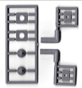
THIS IS A RIGHT ANGLE VENT FOR COMING OUT OF THE SIDE OF A STRUCTURE. IT INCLUDES THE VENT PIPE, FLASHING & TAPERED STACK CAP. PIPE IS 16" DIAMETER BY 3' x 5'. THE END OF THE PIPE IS HOLLOW. PIPE CAN BE EXTENDED WITH KIT 8293. PARTS ARE INJECTION MOLDED IN GRAY STYRENE.
