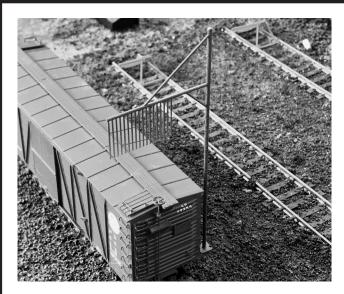
TELLTALES WERE USED TO WARN BRAKEMEN AND OTHERS ON TOP OF CARS OF APPROACHING LOW CLEARANCE CONDITIONS. THEY CONSISTED OF A SET OF ROPES OR CHAINS HANGING FROM A CROSSBAR PLACED SOME DISTANCE BEFORE THE HAZARD. THE ERA IS 1900 TO 1965. HOWEVER SOME ARE STILL STANDING TODAY. THIS KIT IS MOLDED IN STYRENE AND REQUIRES NO ASSEMBLY.
