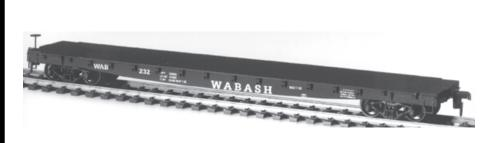
These cars were built from one piece castings supplied by the General Steel Casting Corp. All the RR added was a deck, trucks, brake gear and safety appliances. Because of their one piece design, these cars were extremely long lived. Most RR's had them. This is a beginners kit and does not include brake gear as it is not visible.
