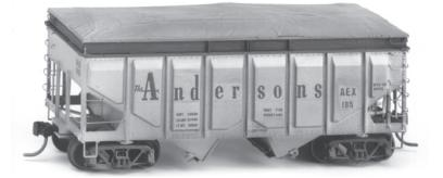
This car is represenative of a series of 114 cars (#'s 131 to 244) acquired by The Andersons Company in 1961 and used in grain transport. Since grain was lighter than coal, the sides were extended to increase the cubic capacity. A canvas cover protected the grain. A cast resin top and custom decal are included. These cars were painted silver and based in Maumee, Ohio. The last ones were retired in 1983.
