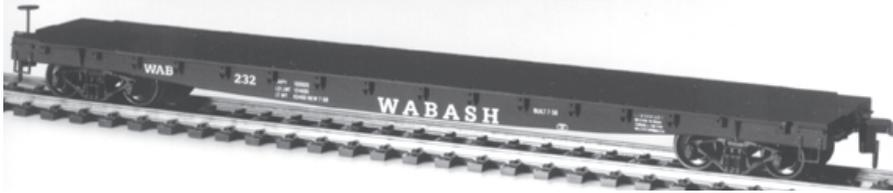
These cars were built from one piece castings supplied by the General Steel Casting Corp. All the RR added was a deck, trucks, brake gear and safety appliances. Because of their one piece design, these cars were extremely long lived. Most RR's had them. This is a beginners kit and does not include brake gear as it is not visible.
