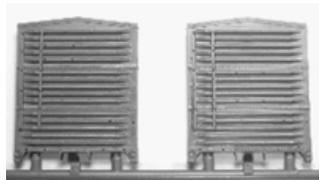
THIS IS A REBUILT 5/5/5 END FOR USRA SS STYLE CARS REBUILT WITH STEEL SIDES. IT HAS AN EXTRA FLAT TOP PANEL AND WIDTH EXTENSION PANELS. THESE CARS ARE 9' 10" WIDE WITH 10' HIGH SIDES. MOLDED IN GRAY STYRENE.
