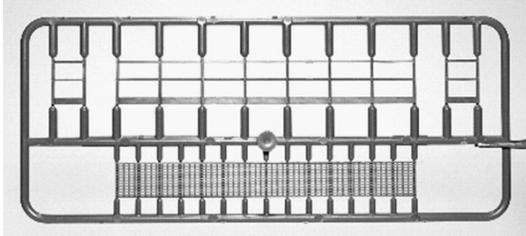
THIS IS AN OPEN GRATE PLATFORM AS USED ON INDUSTRIAL BUILDINGS AND STRUCTURES. IT MEASURES 3/8" x 3-3/8" AND IT INCLUDES THE HANDRAILS. IT IS MOLDED IN GRAY STYRENE.
