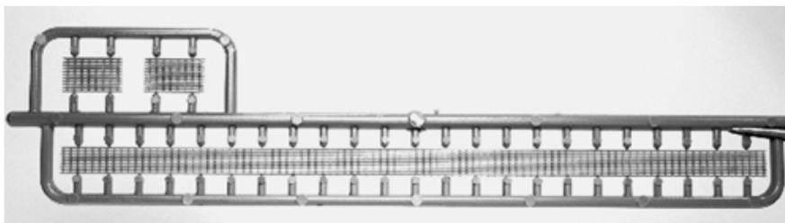
THIS IS A STEEL GRATE ROOFWALK MOLDED IN GRAY STYRENE WITH SCALE SEE THROUGH OPENINGS. IT IS SUPPLIED IN 40' LENGTHS WHICH CAN BE JOINED FOR LONGER CARS. IT WAS FIRST USED ON FREIGHT CARS IN THE LATE 30'S AND WAS THE STANDARD ROOFWALK MATERIAL WHEN THEY WERE DISCONTINUED IN THE 60'S. IT CAN ALSO BE USED ON INDUSTRIAL STRUCTURES.
