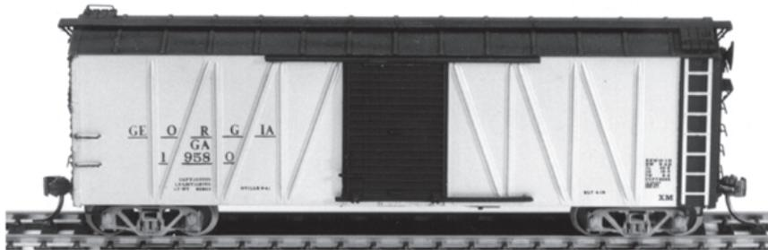
The Georgia RR and several other railroads chose to upgrade their USRA SS cars with steel plates welded to the inside of the bracing in place of the original wood. This was a quick and inexpensive method of obtaining an all steel car. It did not increase the interior capacity as much as the Youngstown sides and ends. AB brakes are included. "D" versions include a Georgia RR decal.
