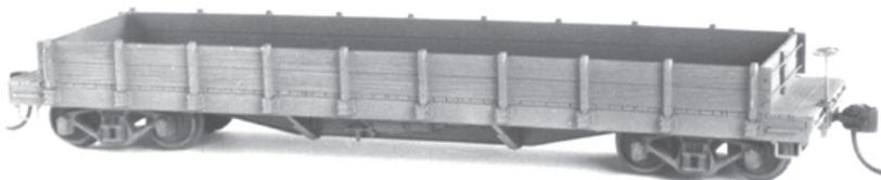
In 1917, 1000 40 foot, 40-ton steel frame flat cars were built for the ACL RR to a standard design with 10 stake pockets. (4021 is the later 50 ton design with 11 stake pockets) Similar cars were built for most RR's. Many were converted to low side gondolas by the addition of stakes and planking. You can build the kit as either a flat or the gondola. "D" versions include an ACL decal.
