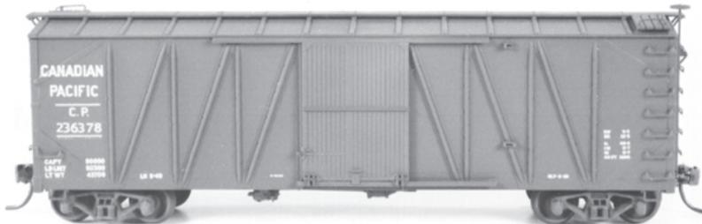
In 1921, the Canadian Pacific RR built a fleet of 3500 SS USRA copies. They were identical with the USRA standard except for the use of 7/8 ends instead of the 5/5/5 end. As built, they had grain unloading hoppers under the doors, but these quickly disappeared. This kit represents the post 1940 version with no grain doors, AB brakes, 7/8 ends and Bettendorf trucks. A CP decal is included.
