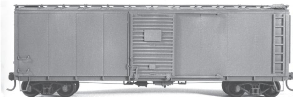
These cars were rebuilt during the late 30's through the 40's from USRA single sheath box-cars through the use of standard side assemblies supplied by the Youngstown Company. Includes both ribbed and non-ribbed extended ends. AB brake gear is included.
