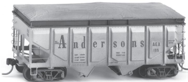
This car is representative of a series of 114 cars (#'s 131 to 244) acquired by The Andersons Company in 1961 and used in grain transport. Since grain is lighter than coal, the sides were extended to increase the cubic capacity. A canvas cover protected the grain. A cast resin top and custom decal are included. These cars were painted silver and based in Maumee, Ohio. The last ones were retired in 1983.
