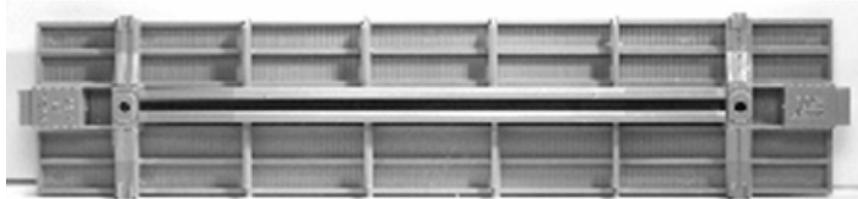
THIS IS THE BETTENDORF STEEL UNDERFRAME USED IN THE REEFER KIT 4024. IT WAS A STANDARD UNDERFRAME ASSEMBLY USED IN THE 20'S & 30'S ON MANY FREIGHT CARS. IT IS INJECTION MOLDED IN GRAY STYRENE.
