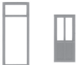
2 LITE DOOR & FRAME 36" W x 80" H .25" x .64" OPENING INCLUDES GLAZING
