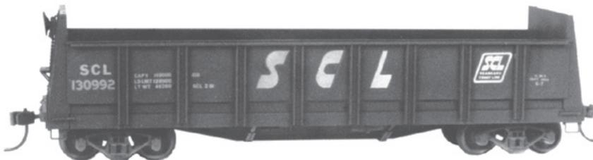
Both the ACL and the SCL converted pulpwood cars into stump cars. These were used used to haul stumps from logging operations to chemical plants that extracted chemicals from the pine tar in them. The conversion was done simply by using steel plates with a pair of angles reinforcing the top edge and channels for vertical support. The gap between the plates and the deck allowed debris to be swept out easily. "D" versions contain a SCL decal.
