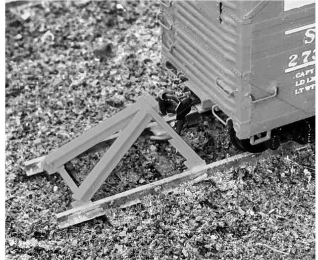
STANDARD HAYES MANUFACTURING CO CAR BUMPING POST. IT WAS FIRST MADE IN 1926 AND CONTINUES IN USE TO THIS DAY. IT IS THE MOST COMMON TRACK STOP AND WAS USED ALMOST EVERYWHERE. THE KIT IS MOLDED IN GRAY STYRENE AND INCLUDES THE REINFORCING PLATES PLACED ON THE OUTSIDE OF THE RAILS.
