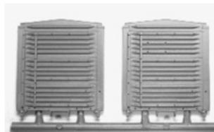
REBUILT 5/5/5/1 END FOR USRA SS STYLE CARS REBUILT WITH STEEL SIDES. IT HAS AN EXTRA 1 RIB TOP PANEL AND WIDTH EXTENSION PANELS. THESE CARS ARE 9' 10" WIDE WITH 10' HIGH SIDES. MOLDED IN GRAY STYRENE.
