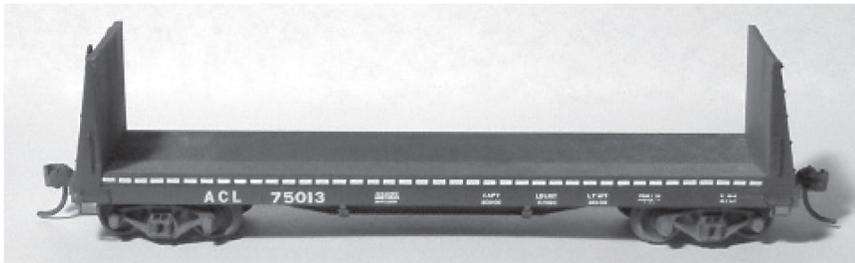
These cars were used to carry pulpwood (small diameter logs of no other commercial value that were used to make paper). They were converted from old flatcars by the addition of a steel deck sloped to the center and bulkhead ends. They were used by the ACL, SEABOARD, SOUTHERN and many other roads that had logging operations in their service area. "D" versions contain an ACL decal.
