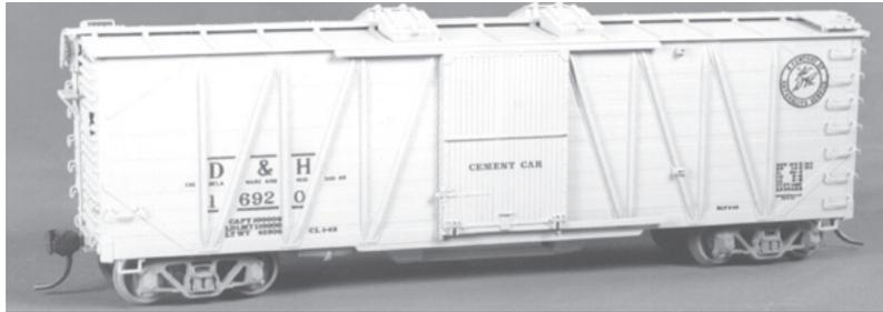
In 1934, the D&H converted 30 SS USRA boxcars to carry bulk cement with the addition of roof hatches, wine discharge gates and interior slope sheets. They were in the # series 17001 - 17500. The B&O also converted 40 cars numbered from 287000 - 287039. After 1960, these cars were used in company sand service with the D&H operating at least one into 1985. "D" versions include a D&H decal, see decal section for B&O decals.
